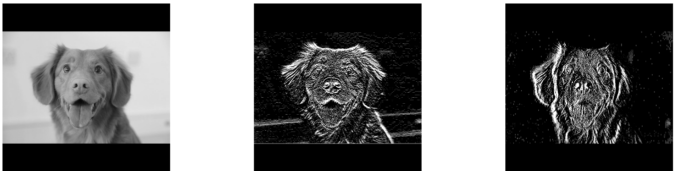
Figure 2: SVD + Discrete Wavelet Transformation. From left to right: Original Image, LH Subband, and HL Subband.
